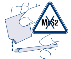
Oil hub and shaft lightly, if necessary ( do not use oil containing MoS2 ).
